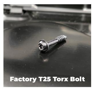
Take the middle torx bolt out from under the MAF sensor and put it aside. It will be used to bolt down the BMS intake bracket to the factory airbox bottom.
