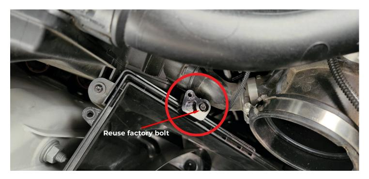
Next loosely bolt the curved "J" bracket to the bracket and BMS intake tube under the MAF sensor. The shorter part of the "J" bracket attaches to the airbox bracket adapter. Longer part to the intake itself.
