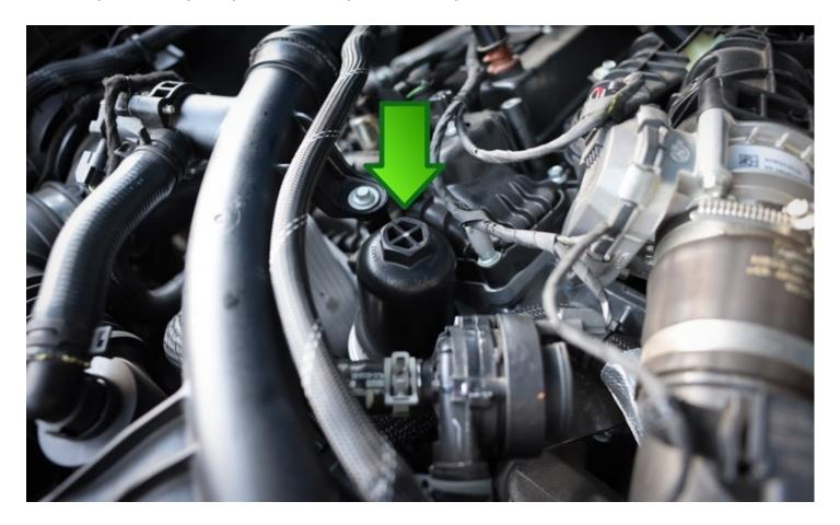
Now remove the inner plastic filter guide/support to the new BMS billet aluminum oil filter cap by carefully grabbing it by the base with pliers and rocking and pulling.
