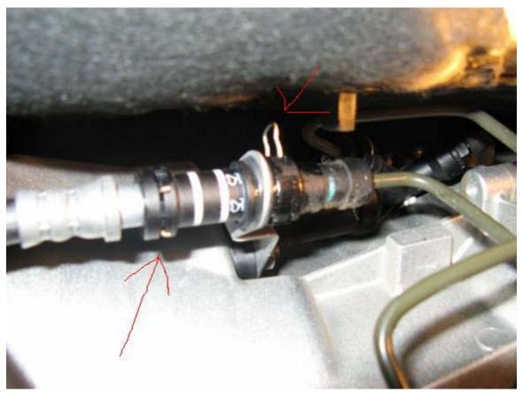
Snap the BMS valve in place, remove the hose clamp, and reinstall the access cover.
