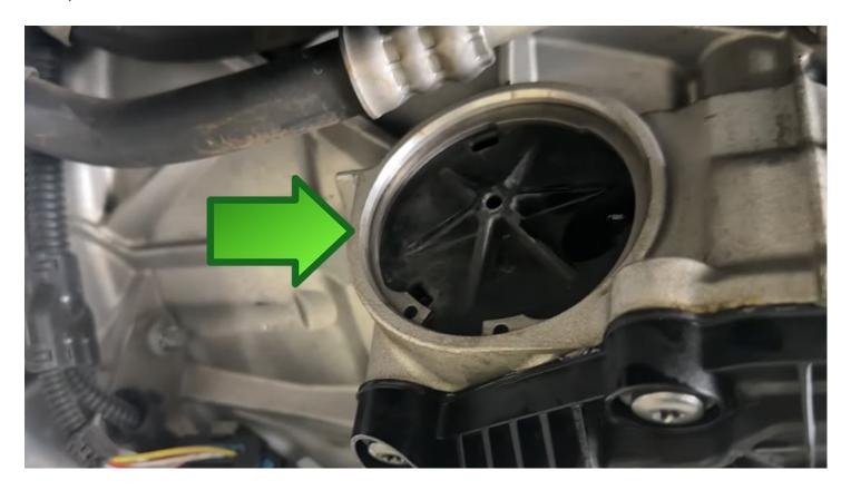
Remove the plastic cover with a hooked pick or similar tool using the oval holes.
