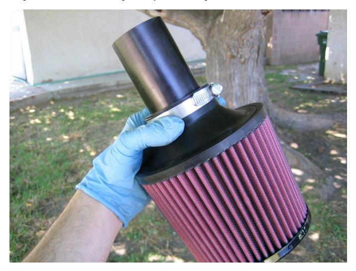
Insert the filter closed to the front of the car first. Slide the intake tube as far in to the factory accordion coupler as it will go, approx 1-2 inches. Tighten clamp.
