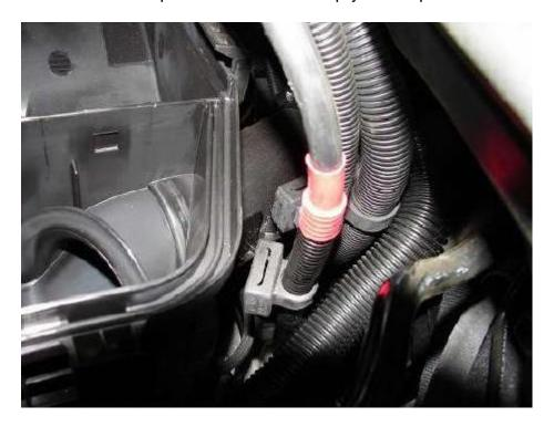
Remove T20 torx screws in the front of the factory cold air scoop.
