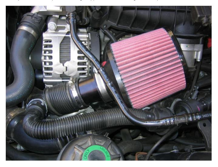
Next position the rear filter. This is the trickiest part of the install process as room is limited and the filter will rub against the front filter and battery cables while being inserted. Stick with it and you'll get it! Having a friend hold the battery cables and front filter out of the way can help. Once inserted tighten clamp.
