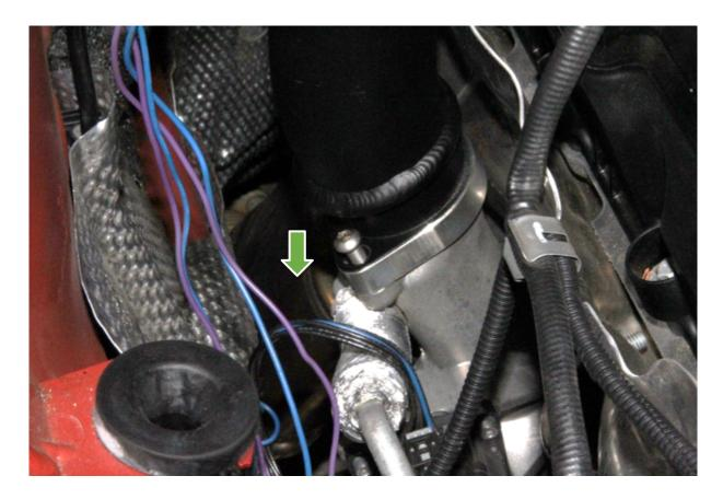
Tighten the clamp on the chargepipe.
