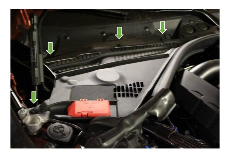
Remove the rest of the bolts from the struts bar and lift it out of the way
