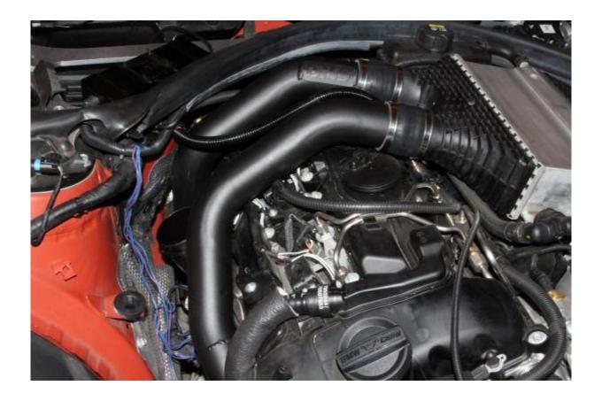
After the chargepipes are installed reinstall the turbo inlet, airbox, strut brace, and associated covers. Installation is complete!
