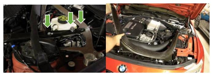
Remove passenger side airbox top and bottom.
