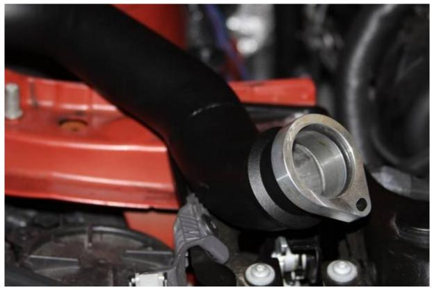
Install the silicon hose on the intercooler and tighten the clamp. Install the chargepipe to the intercooler then to the turbo outlet.
