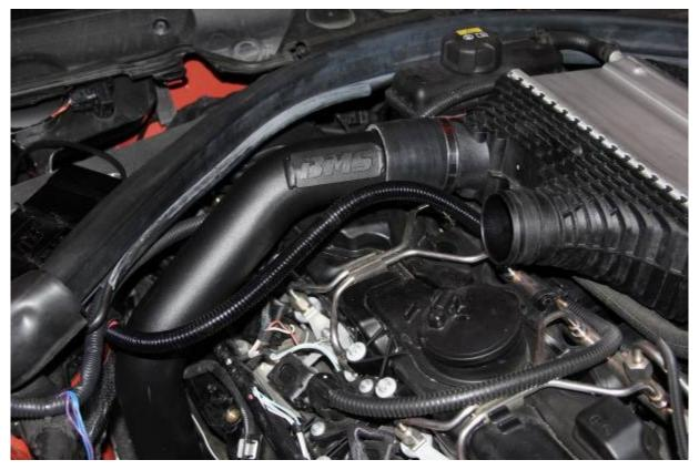
Tighten the chargepipe down with the screws provided with BMS chargepipe.
