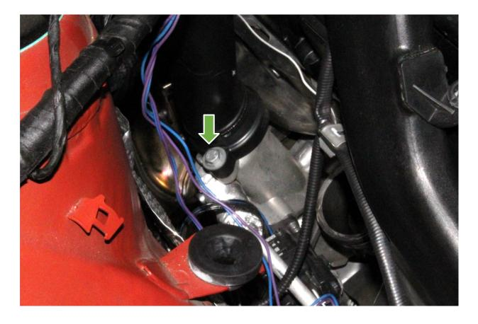
Unscrew the clamps connecting the intercooler and chargepipes.
