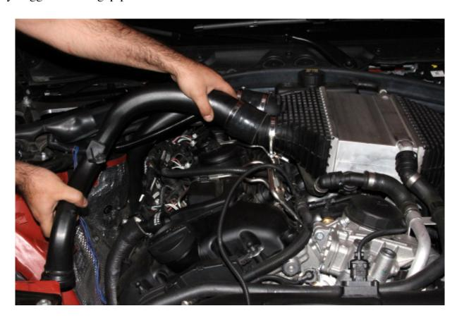
Remove O-ring from OEM chargepipes and transfer to BMS chargepipes.
