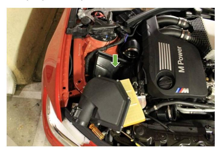
Remove the turbo inlet coupler
