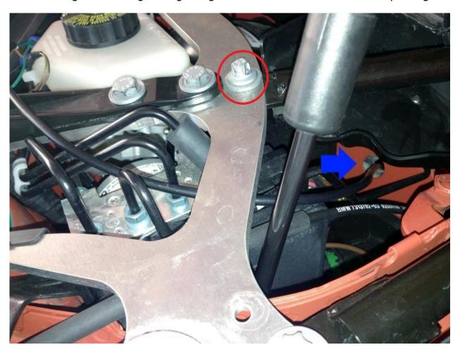
There are two 10mm bolts that you will need to remove to pull the under panel out. Once removed you will see the white wire coming from the grommet hole.
