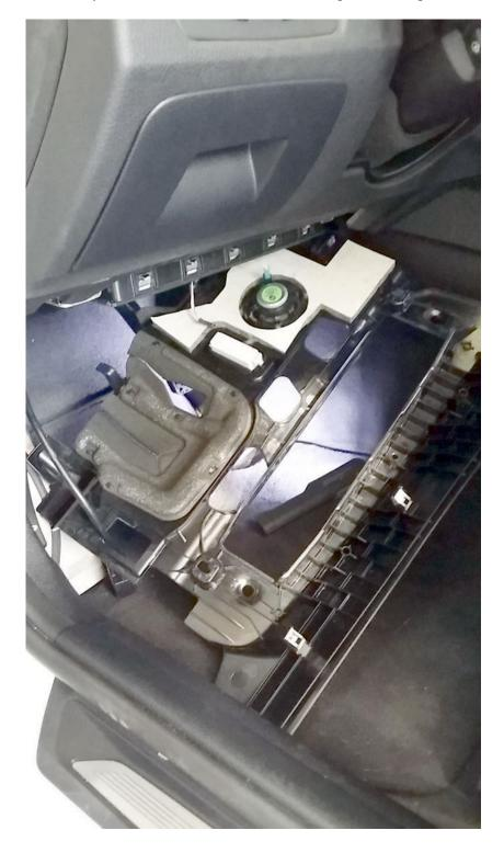
Pull the wire through to where the accelerator pedal sits. Use a T30 bit to remove the pedal bolt and undue the pedal. You will use the provided positap to tap into the white wire (#4).
