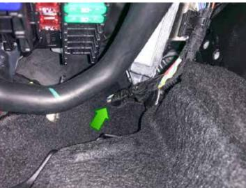
Plug the OBDII wire in to the JB4 green/brown pair connector.
