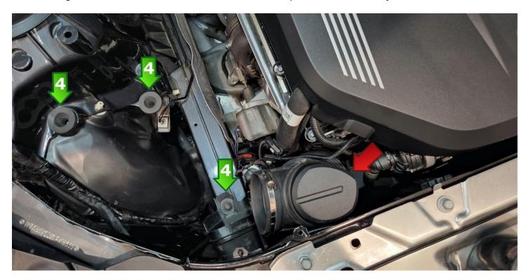
6. Using a T15 Torx tool remove the "MAF" temperature sensor from the factory intake. Place the factory bolts back in the factory intake for safe keeping. They will not be used. Now add the "MAF" sensor to the BMS intake tube using the 2 supplied Phillips head screws.
